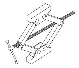
The device is modelled by a rhombus, with each side 25 cm.
